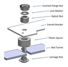
e. Place an included star washer on each post, followed by the flanged nuts, **turned upside down**, and tighten. The flanged nuts must be inverted to provide a catch for the magnetic bracket. NOTE: If your wrench is too thick to tighten the inverted nut, use a tappet wrench or needle nose pliers.
