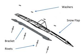
Rivet orientation is critical! Rivets MUST enter from bracket side and out snow flap side. Included rivet washers MUST be used.
